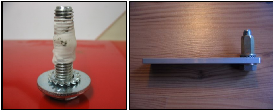
Picture E: Grease applied to the threads of install bolt. (Left) Rivet nut install tool assembled. (Right)
