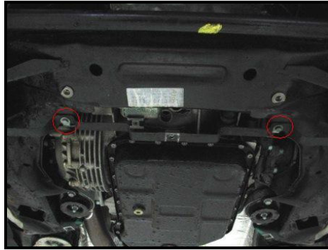
Picture A: Metal bracket that needs to be removed.
