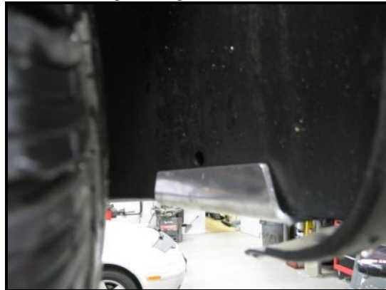
Picture L: Side wing holding the front of fender liner forward.
