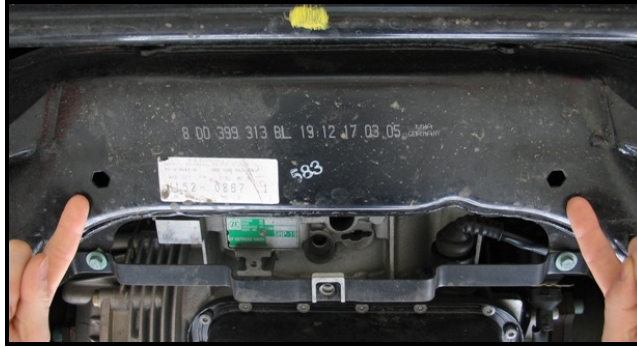
Picture D: Location of where the two Rivet-nuts will be installed on the rear sub frame.
