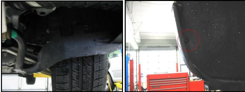
Picture B: Plastic lip that needs to be removed (Left) and Torx screw in the fender liner (Right).
