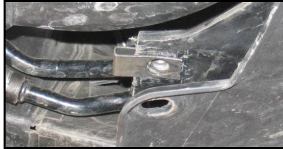
Picture G: 8mm speed clip fully installed.
